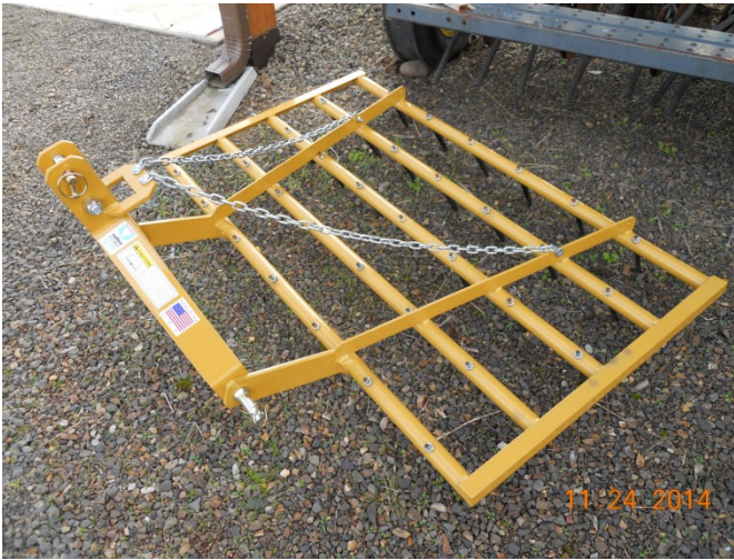
Figure 1: Requires a 20HP tractor minimum with a 3-point hitch and a truck or trailer to transport. Weight 120 lbs. Width 6'.
