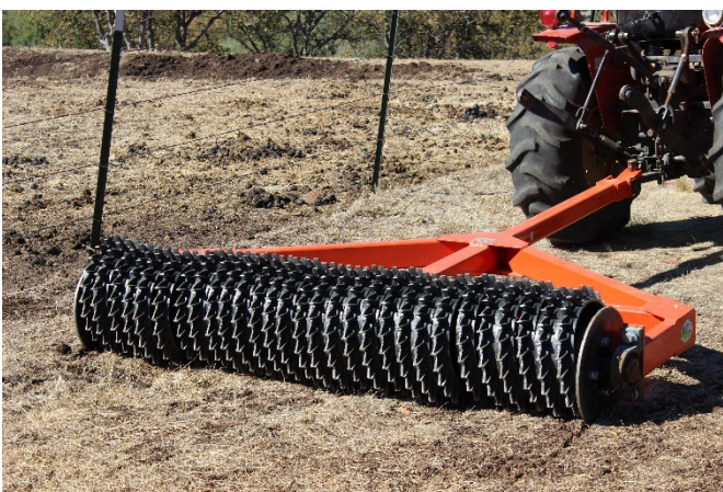
Figure 3: Requires a 18-40HP tractor minimum with a drag hitch and a truck or trailer to transport. Weight 700 lbs. Width 6'8".
