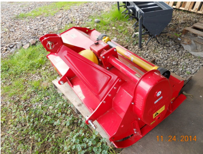
Figure 2: Requires a 20-40HP tractor minimum with a 3-point hitch and a truck or trailer to transport. Weight 485 lbs. Width 6'.
